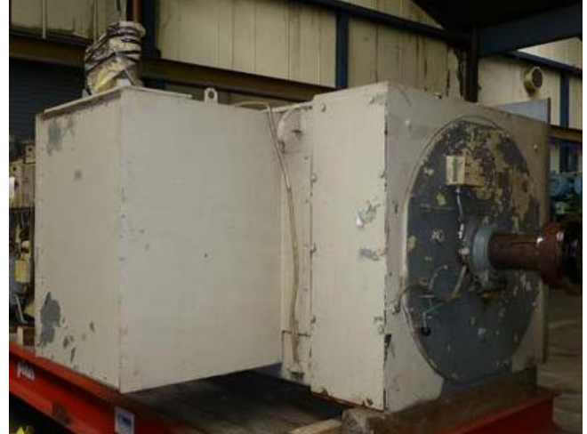
Motor ELIN 60 HZ, 3000 kW/ 4000 HP, 480 A, 4160 V, 1791 rpm
