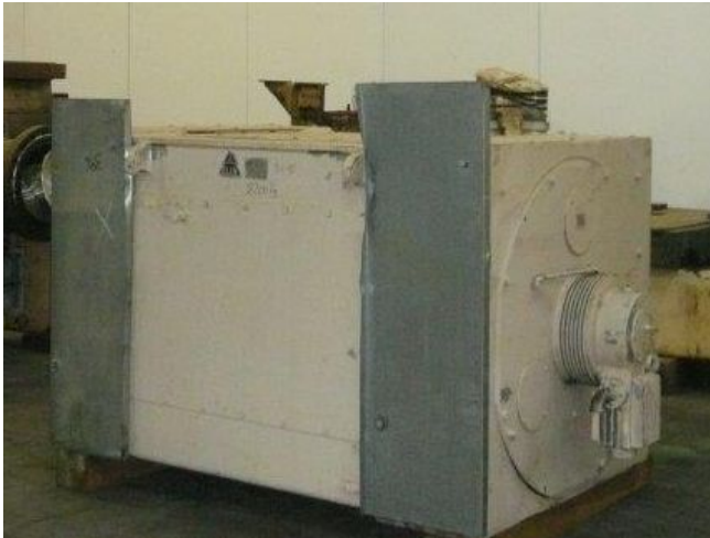
Motor ELIN 60 HZ, 3000 kW/ 4000 HP, 480 A, 4160 V, 1791 rpm
