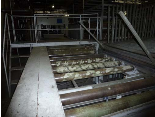
Press outfeed and cooling turner
