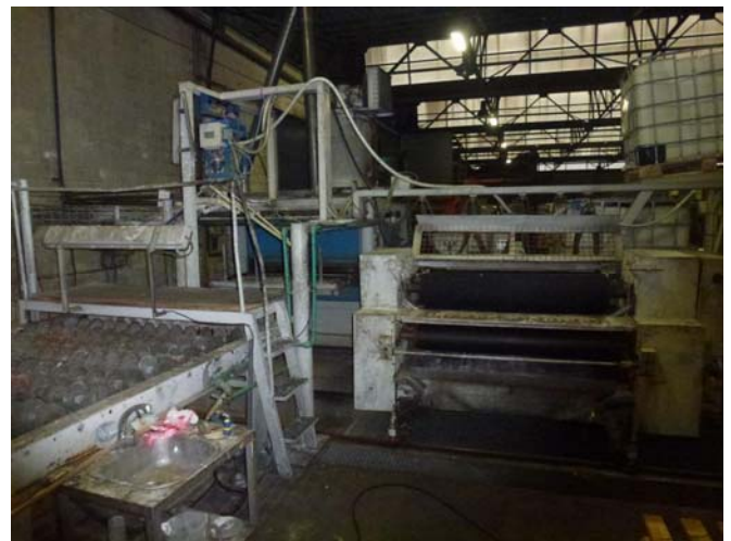
Glue application unit
