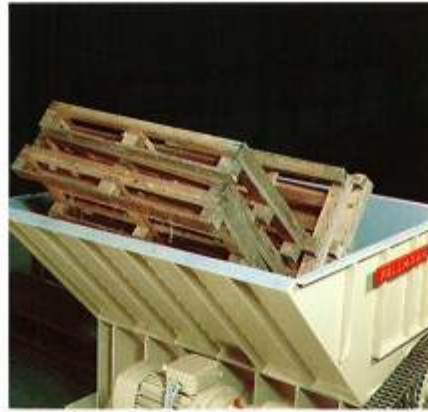
Picture 1: Feed chute of the "Dracula" filled with pallets
