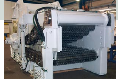
Drum chipper LTH 2000 with entry roller in spike version
