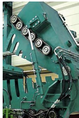
Easily accessible: the wing of the drum chipper in maintenance position
